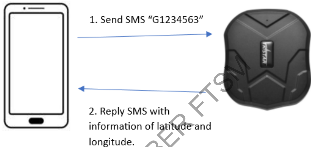
Figure 3.14 Conceptual Diagram of Experimental Setup for GPS Device Tracker
